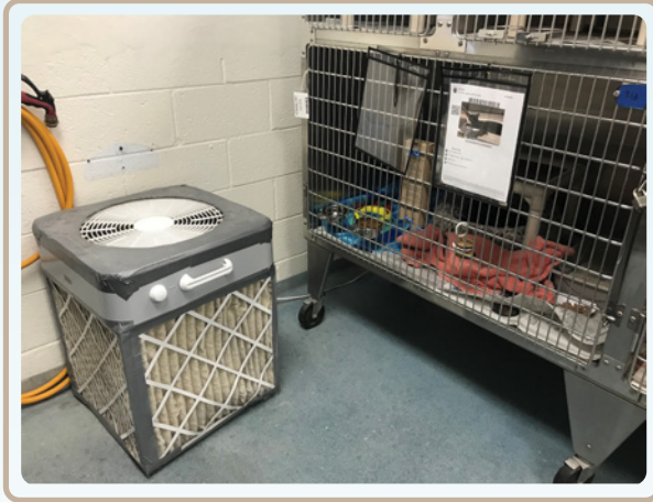
Corsi-Rosenthal Box helping to scrub air in cattery to reduce the risk of cats getting upper respiratory infections
